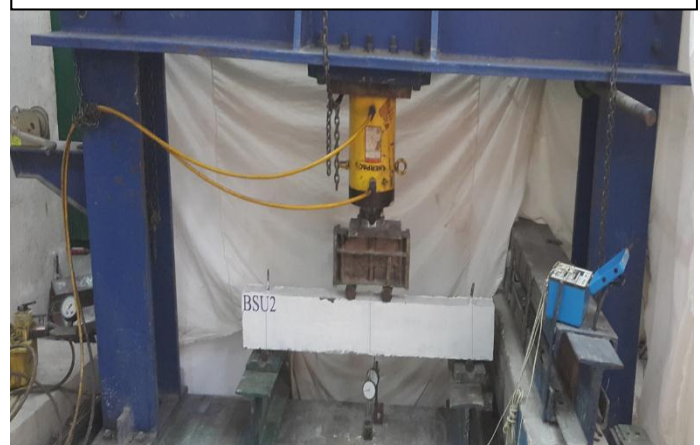
Fig. 2 Test setup of the tested beams.
