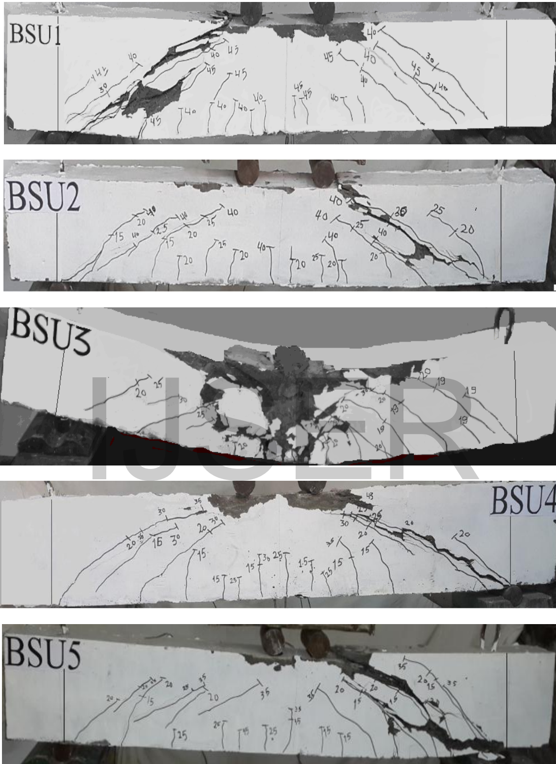
Fig. 3. Photographs of the crack patterns of the tested beams (Note: load marked on the specimens are in tons)
